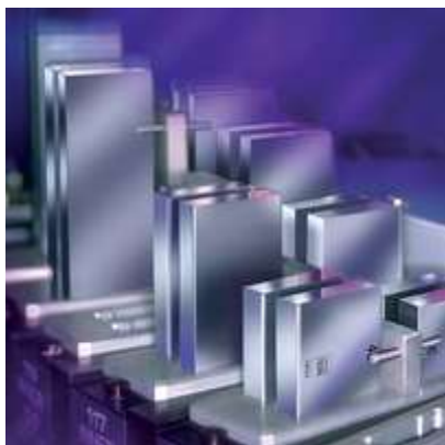
Sets of 11 gauge blocks for the calibration of UPC/UPD gauge blocks comparators
